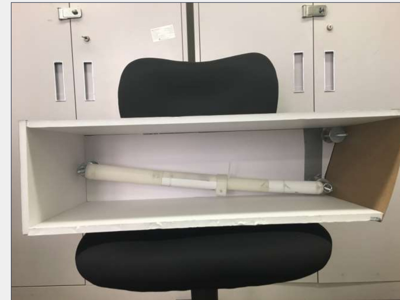
A 3D-printed tie rod hooked up in a mockup space envelope
